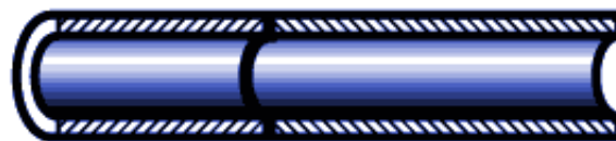
Butt joint - tubular parts (cutaway)
